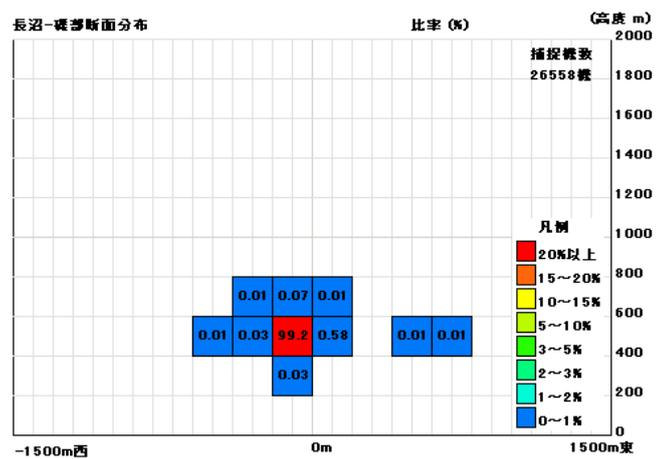
着陸機分散図 (Landing Aircraft Dispersion Diagram)
